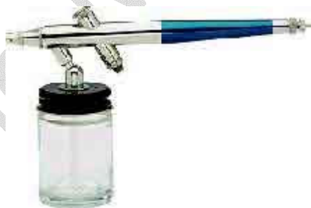
Figure 2 Model 200 bottom feed, single action, internal mix
